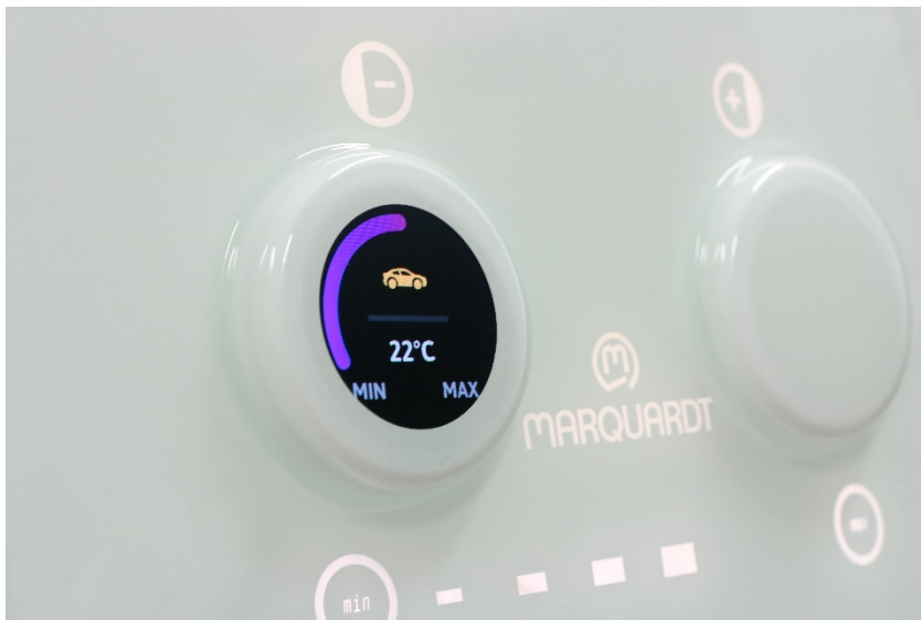
Laser-marked control panel on the backlit touch control unit from mechatronics specialist Marquardt, featured on FOBA's booth at automotive interiors EXPO. (Image rights: Marquardt)
